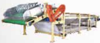
MATRIX CFM (Available in various sizes, from 100kg/hr upto 650kg/hr)
