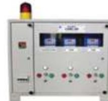
Coal Air Ratio Controller (CARC-04)
