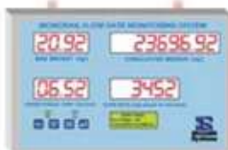
Monorail Flow Rate Monitoring System (FRMS)
