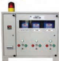
Coal Air Ratio Controller (CARC-04)
