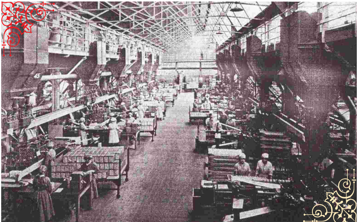
Packeting room, showing twelve automatic units fed from mezzanine hoppers
