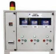
Coal Air Ratio Controller (CARC-04)
