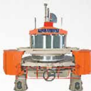
Rollomax Rolling Table (18", 24", 30", 36", 46" with pneumatic automation)
